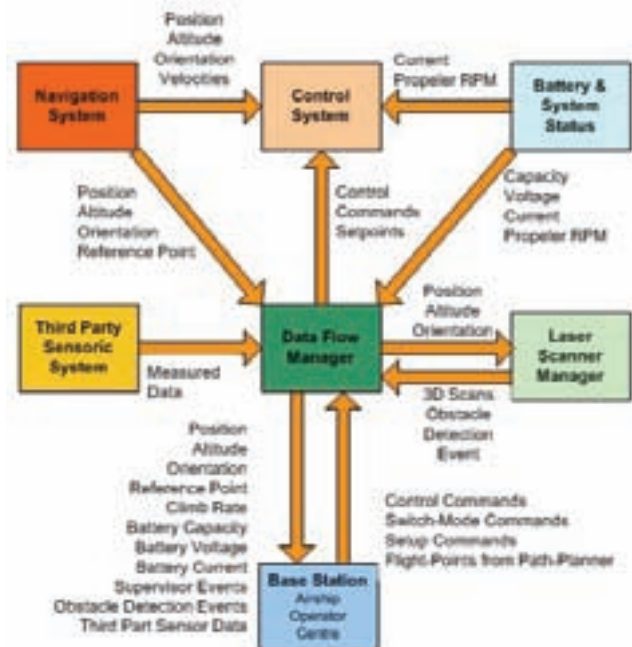
Fig. 6 Schematic of the data relations between the system components.
