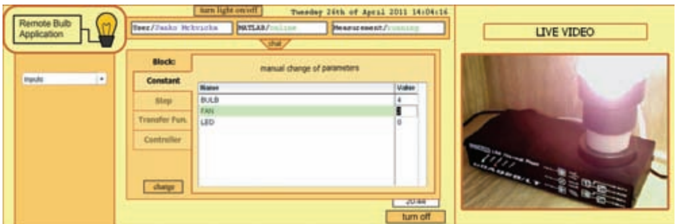
Fig.7 Running experiment (input form where user can change parameters in real time)
