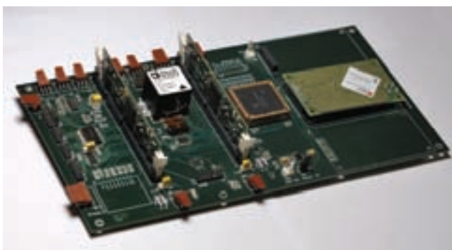
Fig.1 Electronic board of the navigation system (design by Dr.-Ing. Ivan Masár).
