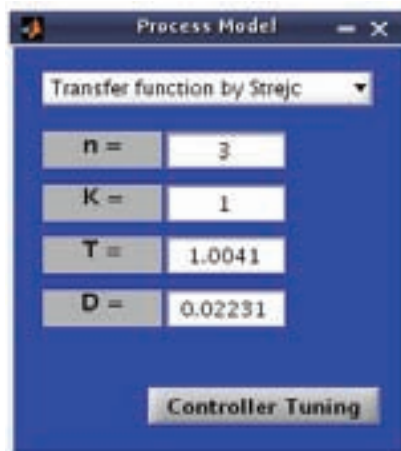
Fig. 8 Identified parameters of aperiodic system
