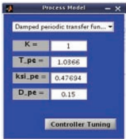
Fig. 9 identified parameters of damped periodic system
