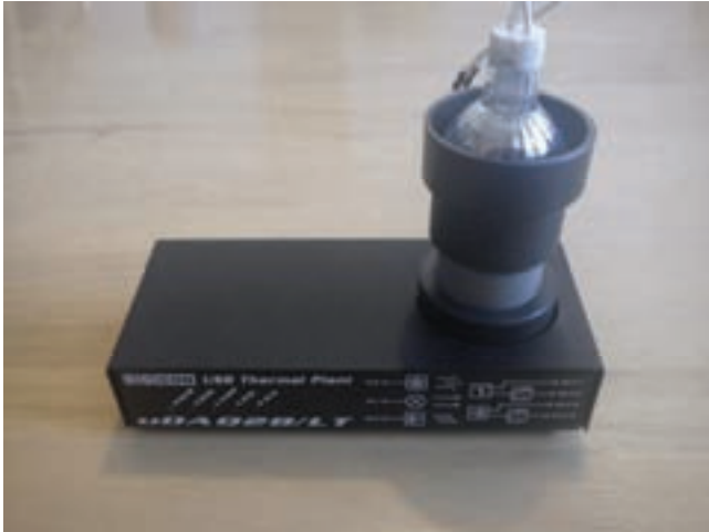
Fig.1 Thermo-optical device uDAQ28/LT
