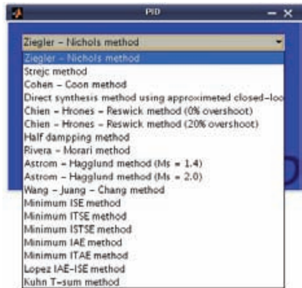
Fig. 16 List of analytical methods used for PID controller tuning
